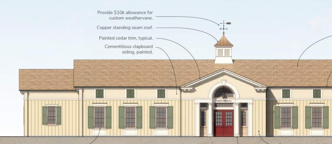
Option A: Aluminum-clad wood – windows & commercial grade doors, custom exterior color, factory primed interior, Marvin or equal.
